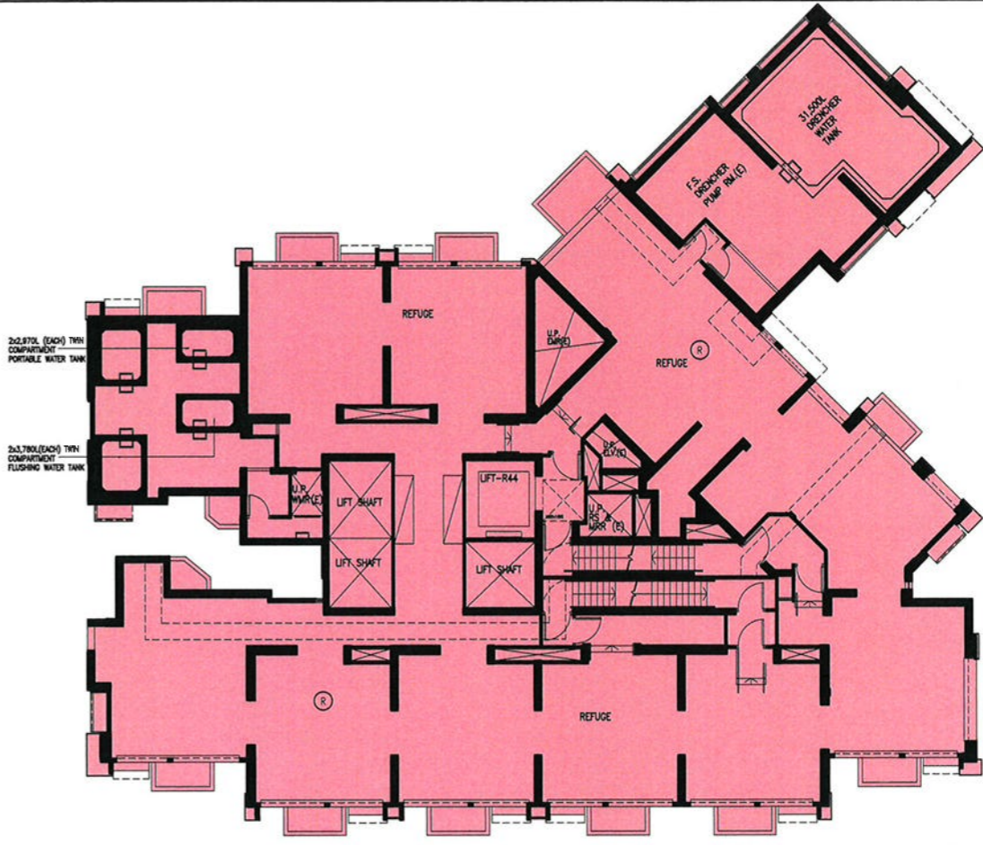
TOWER 7 - 27TH FLOOR (REFUGE FLOOR)
